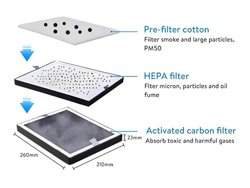
The primary, medium and main filter elements can be replaced separately, which prolongs the service life and reduces the use cost.
